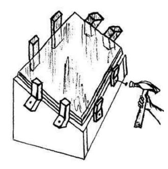
The glass is glued to the top of the box using silicone sealant. If two panes of glass
