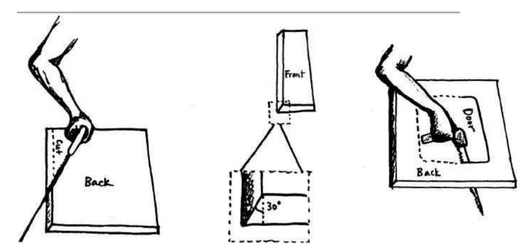
Cut the door out of the back panel.
