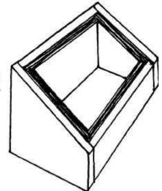
The cardboard and aluminum foil are attached to the interior of the box using nails and large washers.
