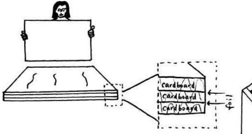
Insulation can be made up of cardboard and aluminum foil.
